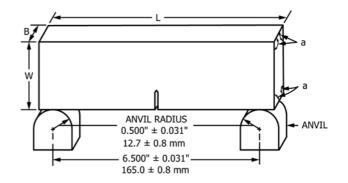
Dimensions and Tolerance for Specimen Blank
